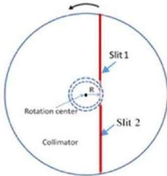
Figure 8 – Optimized Collimator Geometry with Two Off-Axis Slits
