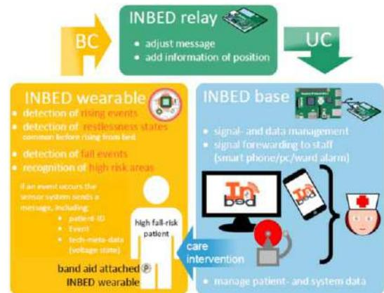
Figure 3– INBED system functionality diagram
