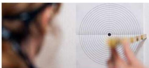
Figure 2 – After 1 minute resuscitation the deviation of calibrated eye-tracker was tested with the help of a target disc.
