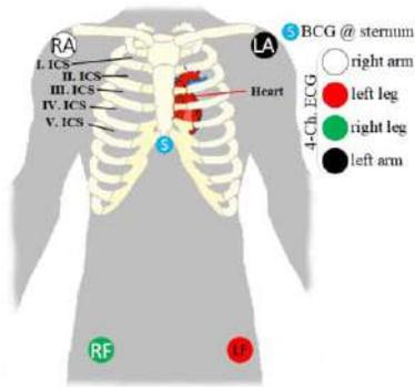
Figure 2 - Sketch of the attached Shimmer 3 ECG Unit (BCG) and the positions of the electrodes on the upper body.
