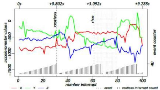
Figure 5– Diagram of the recorded INBED data during rising (raw triaxial acceleration data lines) – in lower area the restlessness counter lines - dashed line show the triggering of the alarms (restlessness and uprising) - grey dotted lines represent standing
