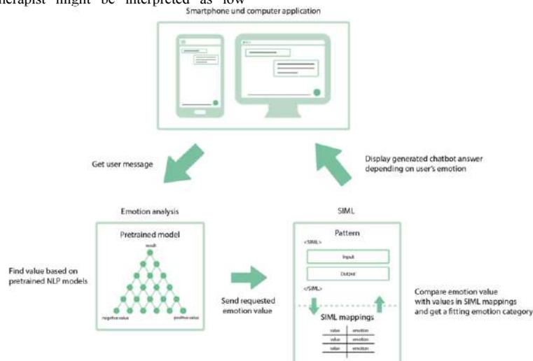
Figure 4: System architecture
