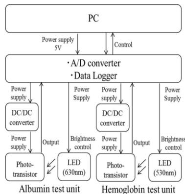
Figure 2 – System Block Diagram
