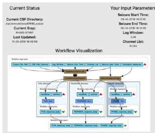
Figure 1 – User interface with visualization of the workflow module status. Light blue boxes are inputs, dark blue are REST calls, and brown are BeanShell scripts.
