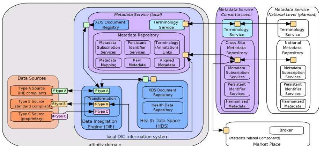
Figure 1– High-level System Architecture of Metadata-related Services at different Levels
