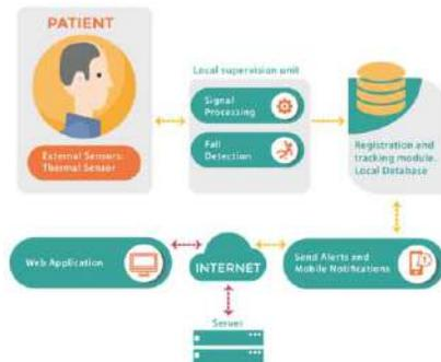
Figure 2 – Thermal Sensor Diagram
