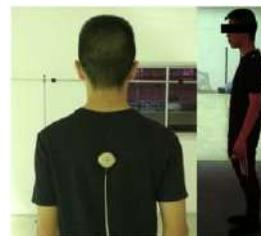
Figure 1— The wearable device containing an accelerometer sensor and vibrotactile biofeedback module was attached to the participant to measure the tilt angles of the body.
