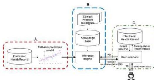
Figure 1-Components of the fall prevention CDSS
