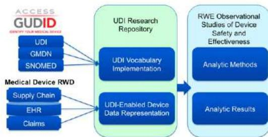
Figure 1. System architecture of our proposed framework. RWD: Real-World Data; RWE: Real-World Evidence.
