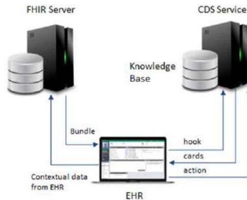
Figure 2 - CDS service architecture
