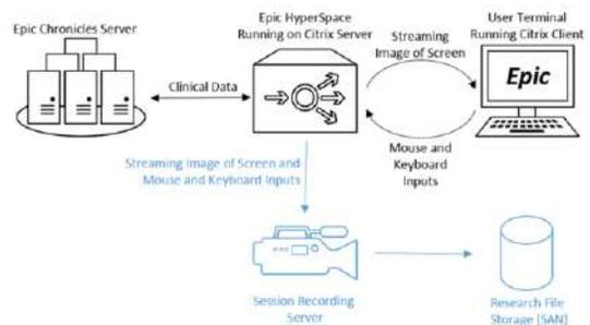
Figure 1— System Diagram of Screen Capture
