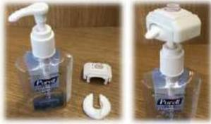
Figure 2 – Disinfection Pump Operation Detection Sensor
