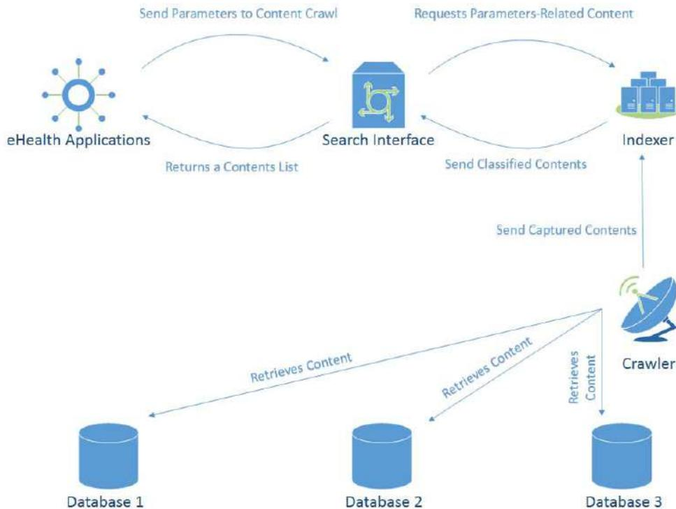
Figure 1. Architecture of Integration System
