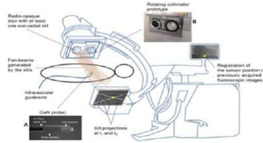
Figure 2 – Implementation of Virtual Fluoroscopy Guidance
