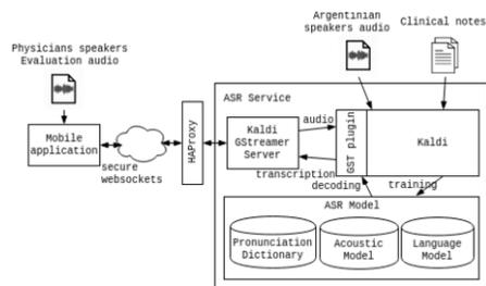
Figure 1– Automatic Speech Recognition (ASR) System architecture
