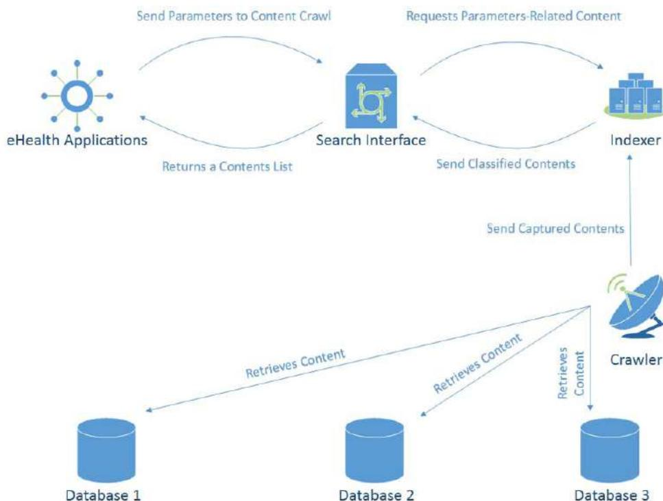
Figure 1. Architecture of Integration System
