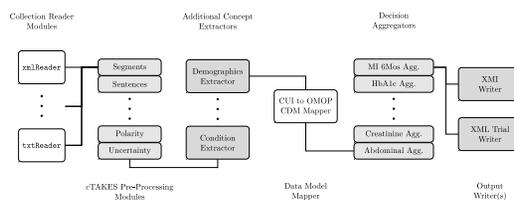
Figure 2 – Six Conceptual Classes of Pipeline Modules in Use
