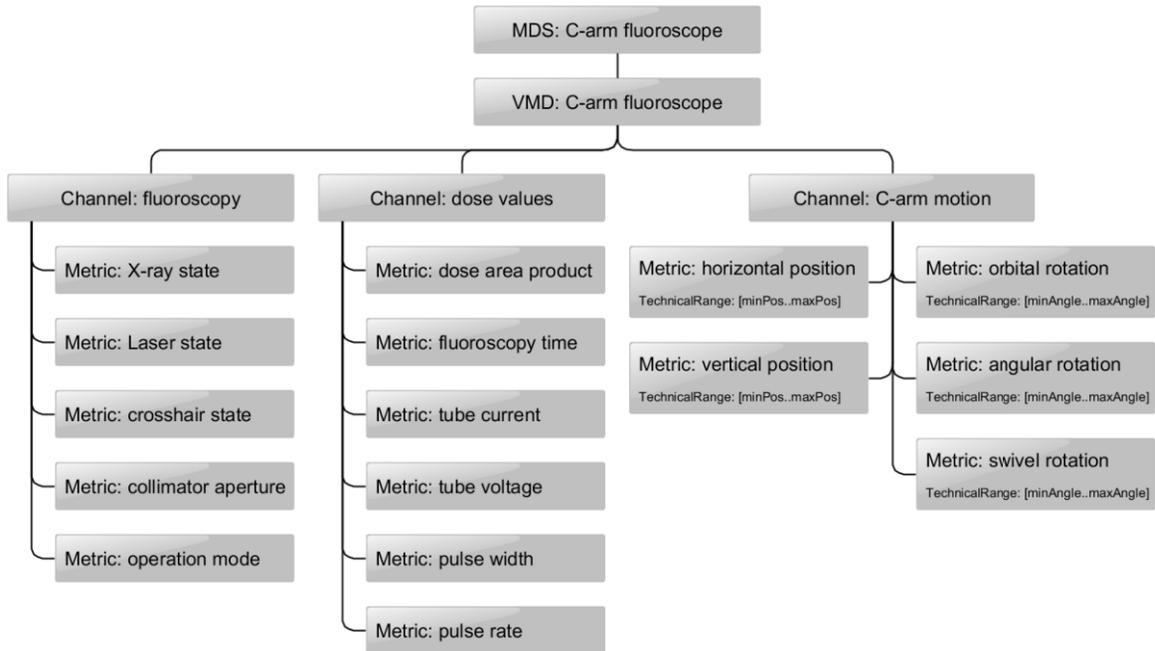
Figure 1 - Simplified model of a C-arm fluoroscope as a hierarchical containment tree; operations, contextual information, and alerts are omitted for brevity.
