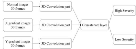
Figure 12 – Work flow for 3D CNN Model
